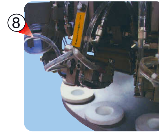
I SISTEMA DI CHIUSURA A PINZE CALDE PER TUBETTI IN POLITENE, LAMINATO E POLYFOIL UK HOT JAWS SEALING SYSTEM FOR PLASTIC, LAMINATED AND POLYFOIL TUBES
