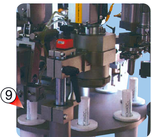
I SISTEMA DI CHIUSURA AD ARIA CALDA PER TUBETTI IN POLITENE, LAMINATO E POLYFOIL UK HOT AIR SEALING SYSTEM FOR PLASTIC, LAMINATED AND POLYFOIL TUBES
